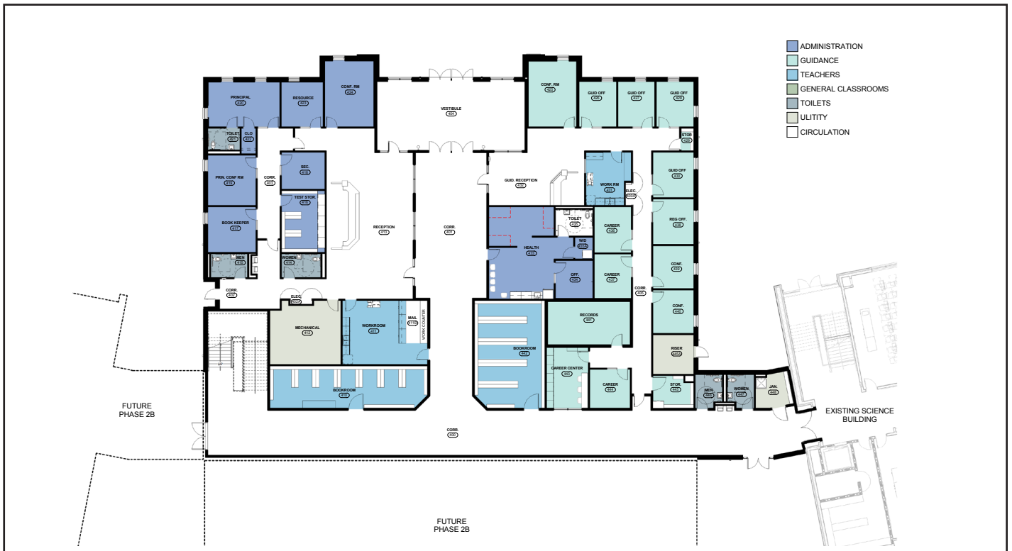
PHASE 2A 1ST FLOOR: ADMINISTRATION AND GUIDANCE
